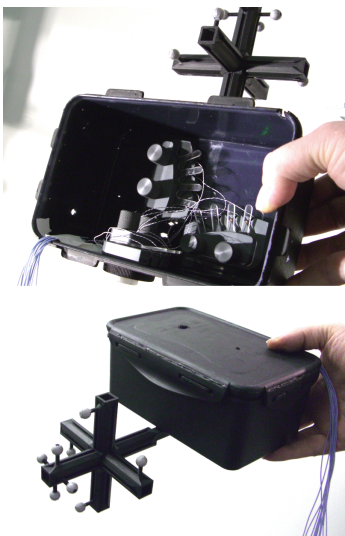
Figure 1: The container with the EMA sensors and OPT markers.
